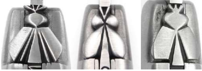
Examples chiseled with a file
